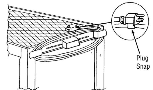
For safety and neat appearance, secure cord plug to cord with plug snap.
