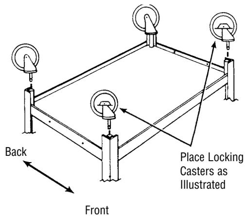
Turn bottom stand assembly upside down on a smooth surface. Push the four casters firmly into the caster socket holes in bottom of each leg as illustrated.
