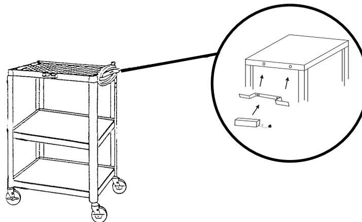
Place metal cordwrap onto metal top shelf making sure that the holes on the cordwrap align with the holes on the shelf. Place the two screws through the holes of the electrical assembly. Place the electrical assembly with the two screws through the holes of the cordwrap and mounting bracket. Secure screws with wingnuts.
