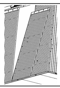
**Note:** To remove a Wall Panel, slide it to the left (when looking at it from inside the shed) until it lifts out.
