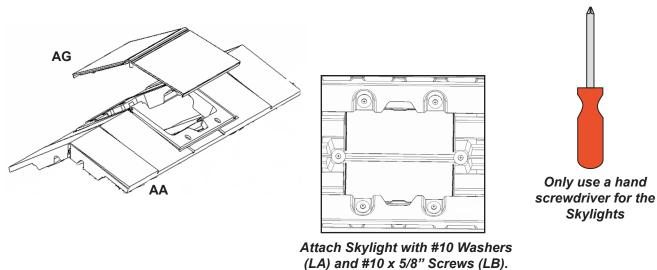
Opt. 2.17: Install both Center Roof Caps (with Skylights) onto the shed.
