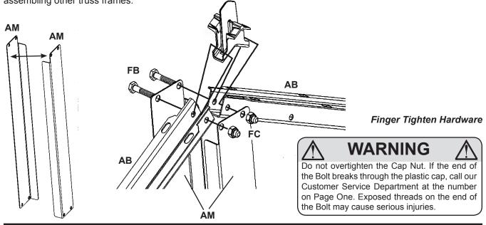
Opt. 2.11: Attach a Gutter Channel (AB) (Truss Support Strips (AM) fit inside Gutter Channel (AB)). Attach Truss Channel (AD) to Gutter Channel (AB) at each end.
