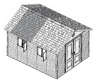
**Note:** Your shed may be shorter than shown above. Skip the very back Roof Panels (slightly more narrow than the middle Roof Panels) and then remove the next two Roof Panels from each side of the shed (along with the connected Roof Caps).
