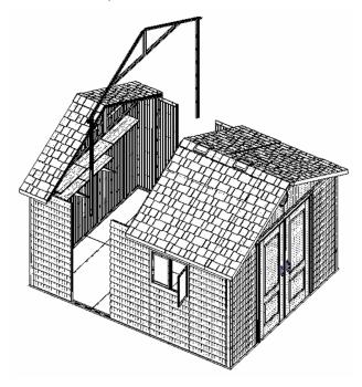
**Opt. 2.6:** With at least on person on each side of the shed, tip the back section of the shed forward to about a 45 degree angle and slide the back section away from the shed..
