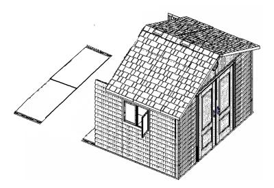
**Opt. 2.9:** With at least on person on each side of the shed, tip the back section of the shed forward to about a 45 degree angle and slide it forward to re-connect it to the rest of the shed.
