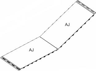
Opt. 2.8: Connect the Inner Floor Panel extensions (AJ) to the other Inner Floor Panels on the main section of the shed.
