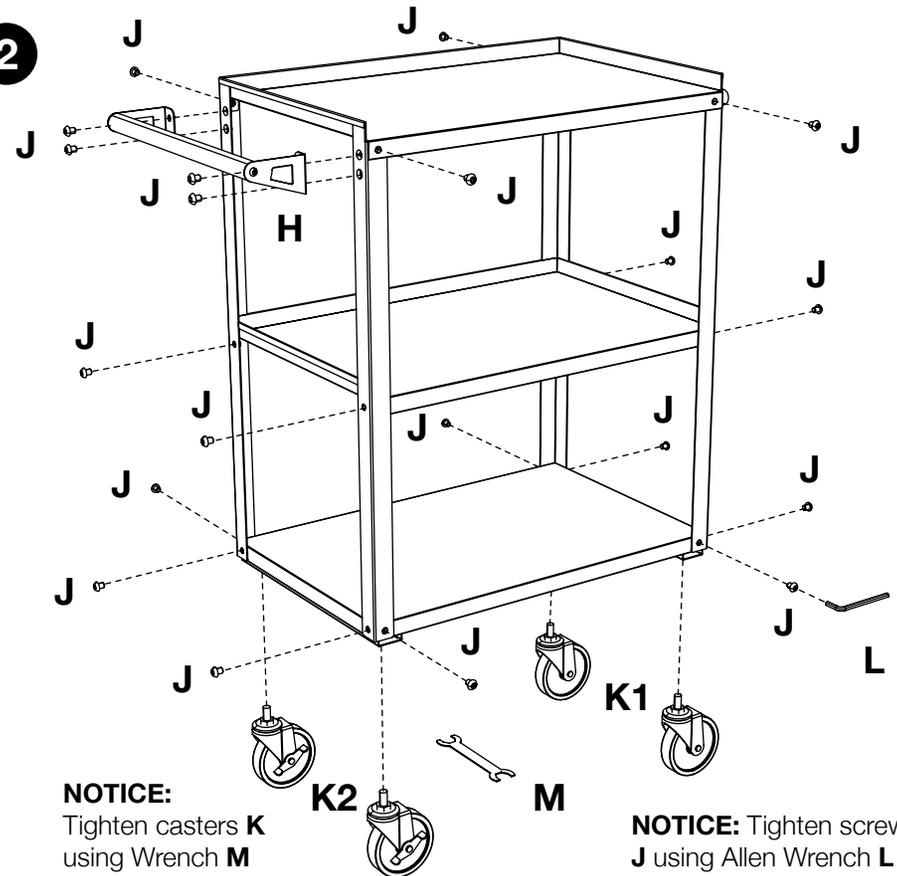
**NOTICE:** Tighten casters K using Wrench M
