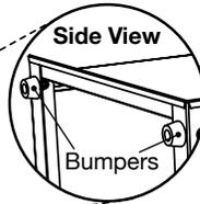
**NOTICE:** Legs with bumpers must be installed on the opposite side of the handle
