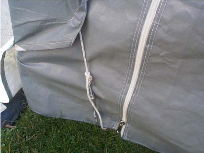
**Step 3.** When the cover is completely aligned secure the cover to the bottom tie-down cross rail using the rope provided. Start at one end and tie off the rope to the cross rail. Lace the rope through the grommets in the cover and back under the tie-down cross rail. Repeat this on the opposite side
