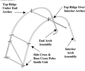
**Step 5**. Begin the Top Ridge Rail by placing a Swedged Cross Rail <u>underneath</u> the End Arch Tube. Secure the Cross Rail loosely with a Carriage Bolt#CBN-3000-2 with washer and nut facing the interior of the unit.
