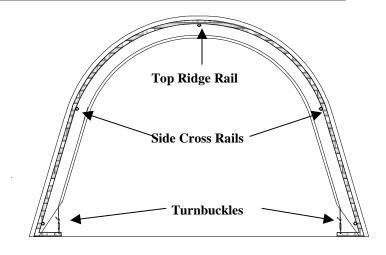
Note: Adjust the end door panel by turning the turnbuckles or repeating step 3 on a regular basis
