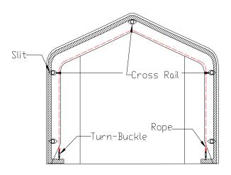
Note: Adjust/Snug the end panel by turning the turnbuckles or repeating step 3 on a regular basis
