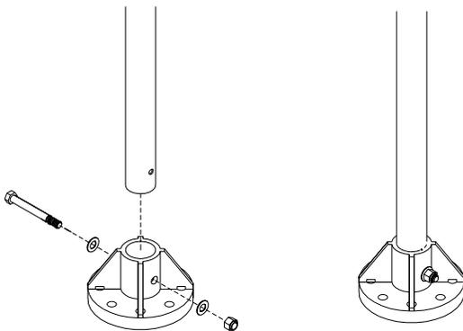
Insert the leg poles (#2) into the white plastic foot plates (#12) so that the base holes align with the corresponding
