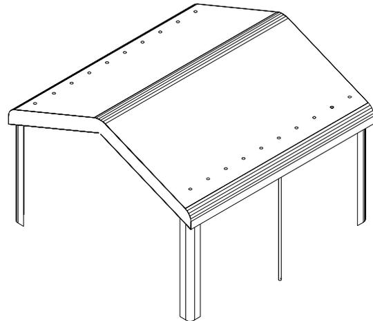
Part of the roof cover extends down each of the 4 corners and attach to the poles by way of the "S" shaped hooks that locate in pre-drilled holes of the Corner Poles.
