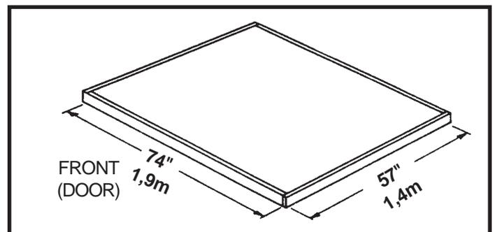
Note: Finished Slab dimensions, with lumber removed.
