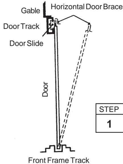
**3** Fasten the door to the door slides using a #10Bx1/2" screw.
