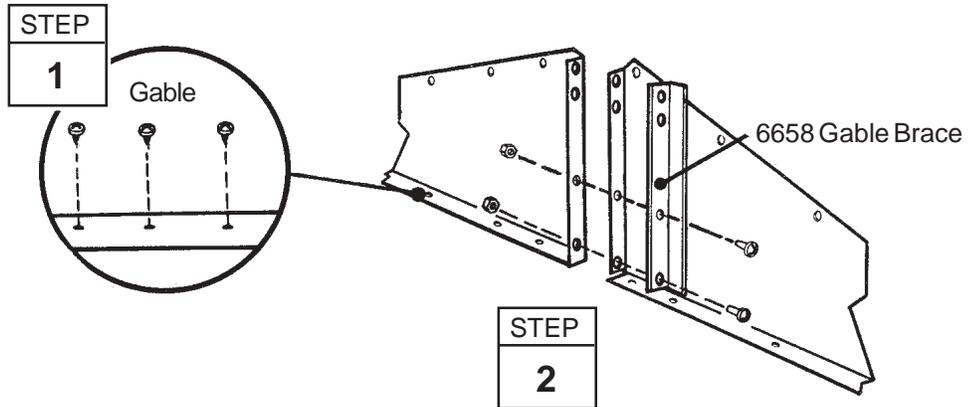
**1** Lift and fasten a right and left gable, under angle at corner, to the door track with screws.
