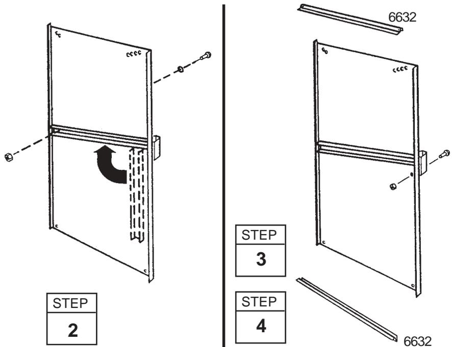
**5** Attach the **lower door guides** as shown.
