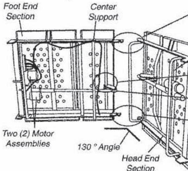
5. Hook the TOP center mounting latch on the HEAD end section of the bed with the TOP center mounting rivet on the FOOT end section of the bed.
