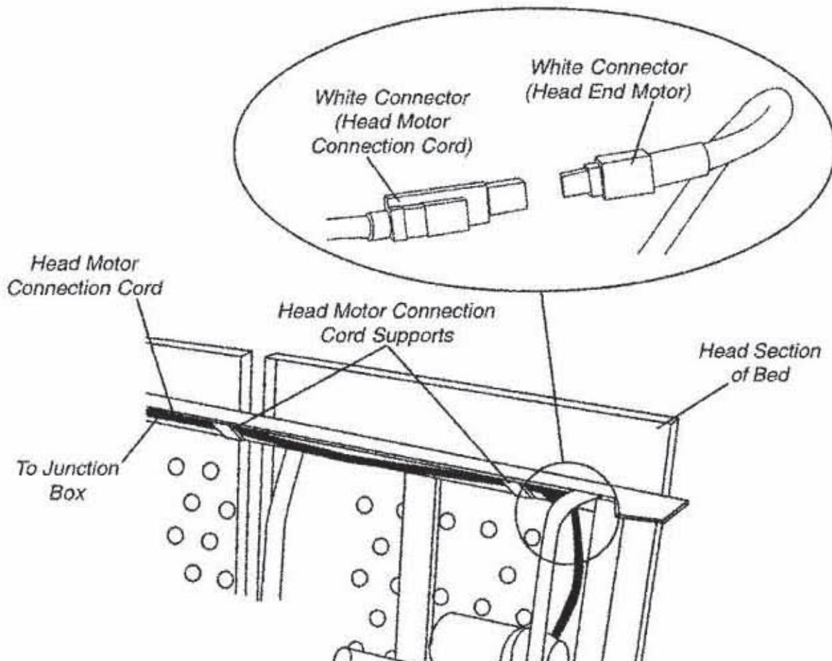
CONNECTING THE HEAD END MOTOR TO THE JUNCTION BOX
