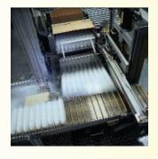
Medline produces 1.6 million medicine cups every 24 hours (64 cups every 3.5 seconds) using the world's most advanced manufacturing system of its kind. The entire system converts (from) plastic pellets to molded, stacked, poly sleeved, and boxed medicine cups automatically. Each operation is electronically verified.
