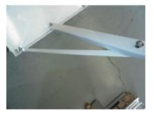
4. Repeat above step by setting the BT-FL-STAND-CROSSBAR diagonal to the BTFL-STAND-CROSSBAR inserted in the above step. This is shown below:
