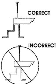
Drill and fasten wood to steel frames using dry wall screws.
