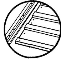
Be sure that you have the correct panel in each position. Do this by overlapping the panels and determining if the holes line up with the holes in the frame.
