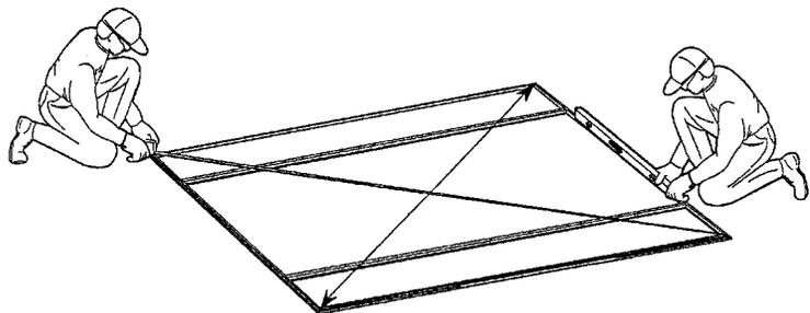
**FRAME MUST BE SQUARE AND LEVEL BEFORE ATTACHING PLYWOOD.**
