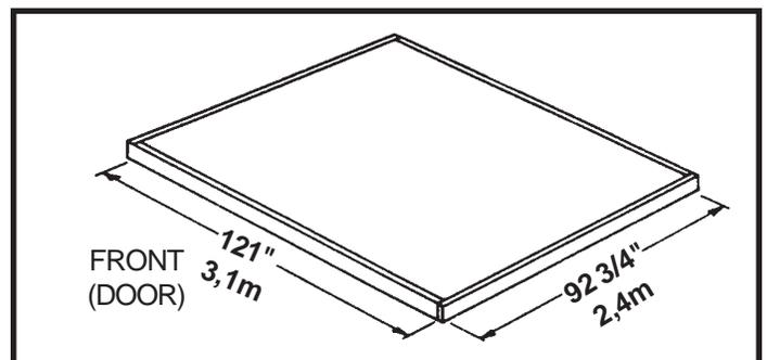
**Note:** Finished Slab dimensions, with lumber removed.
