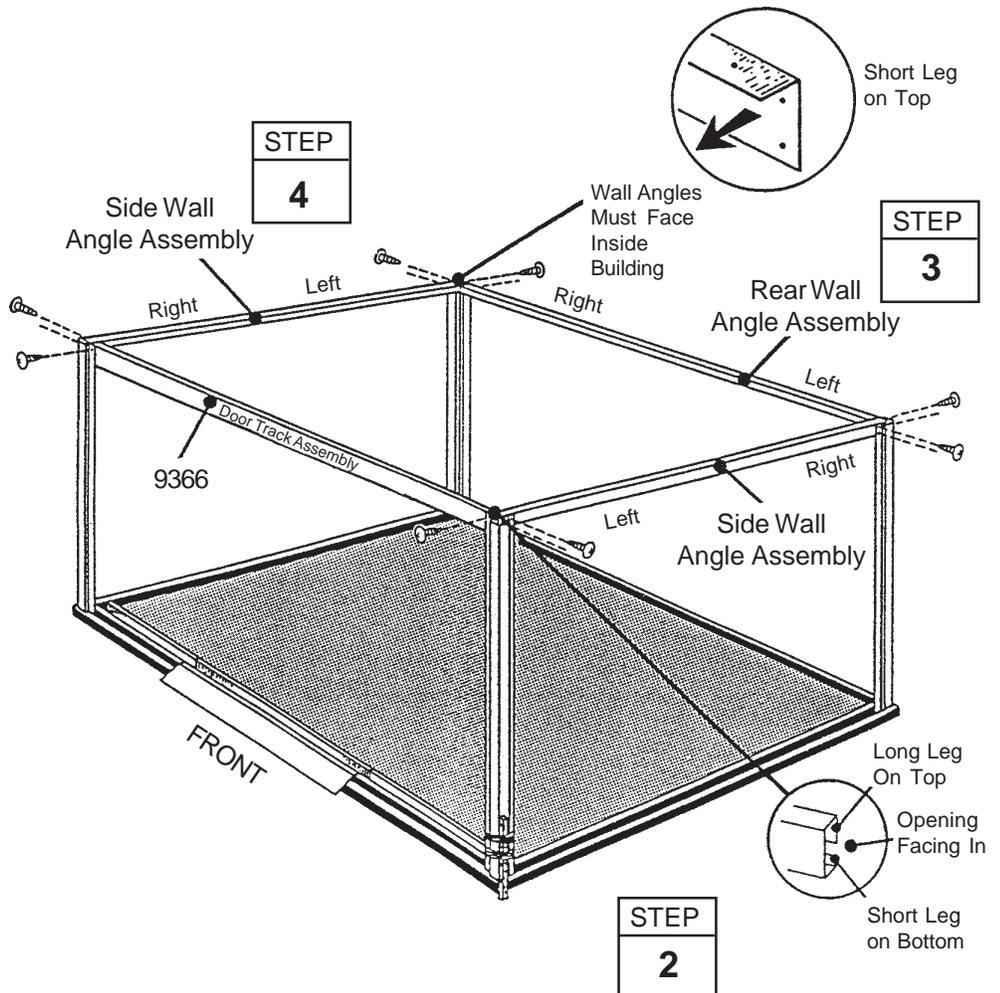
**The floor frame *must be square and level* or holes will not align.**
