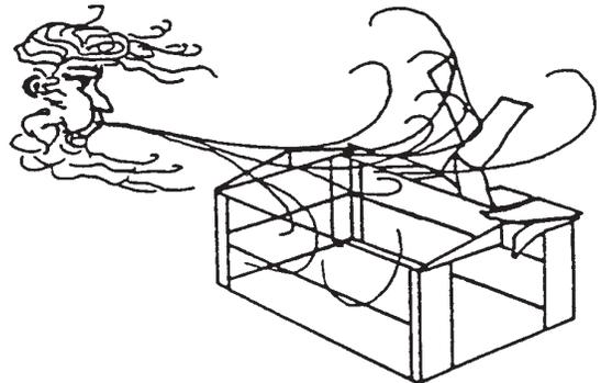
•Do not attempt to assemble the building on a windy day, because the large panels acting as a "sail", can be whipped about by the wind making construction difficult and unsafe.
