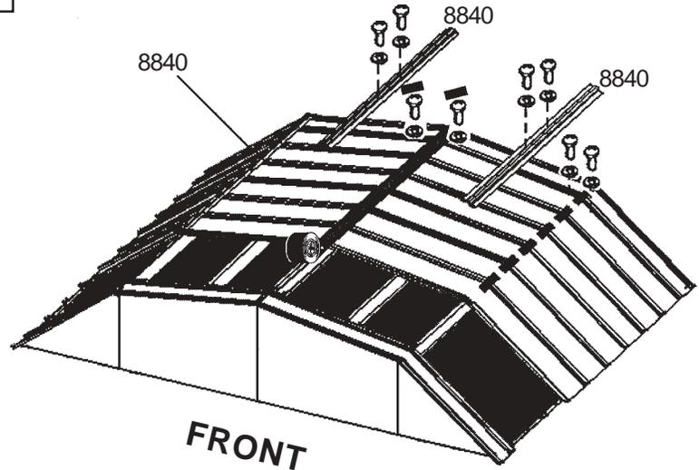
**2** Install the second **ridge caps** overlapping the first ridge caps while installing the remaining narrow **roof panels**. Cover the notched areas of the roof panels with strips of weather stripping tape and continue weather stripping the ridge.
