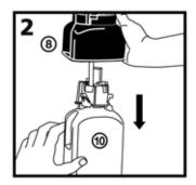
While still pushing the Green release latch, pull downward on the Refill Bottle (10) and remove it from the Motor Assembly/Bottle Support (8).
