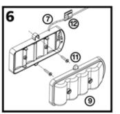
Remove the cover from the Battery Box (9) by loosening the two captive screws on the Battery Box cover. Position the Box on a convenient (vertical or horizontal) surface under the counter top that will allow access for battery changing. Attach the Box to the surface using the two screws (1) and anchors (if attaching to a plaster or masonry surface). Use the Wall Clip (2) to secure the Power Cable (7) to a wall or other under-counter surface if desired.
