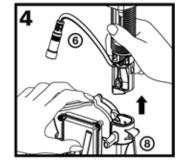
Align the indent inside the top of the Motor Assembly/Bottle Support (8) with the indent on the shank of the Dispenser Assembly (1) and firmly push the Motor Assembly/Bottle Support up, onto the shank.
