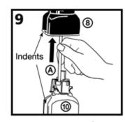
Feed the dispense tube (Å) on the Refill Bottle (1) up through the Motor Assembly/Bottle Support (8) and Dispenser Assembly (1), aligning the two indents in the Bottle and the Support. Slide the Bottle upward until it snaps into place.
