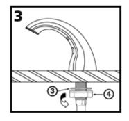
From underneath the counter, first feed the Lock Washer ③ and then the Mounting Nut ④ over the Data Cable ⑥ and onto the threaded shank of the Dispenser Assembly ①. Be sure that the "teeth" on the Washer will touch the bottom of the counter top and that the Nut threads easily onto the shank. (If the Nut is hard to turn by hand, it is upside down.) Hand-tighten the nut securely.
