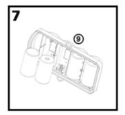
Place four alkaline "D" Cell batteries into the Battery Box (9) cover. The batteries must be positioned according to the diagrams shown on the inside of the cover.
