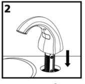
Feed the Data Cable (6) and the shank of the Dispenser Assembly (1) through the hole in the countertop. Point the spout of the Dispenser into the sink bowl and press down firmly on the Dispenser to securely attach it to the countertop.
