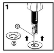
Remove the paper liner from one side of the Adhesive Gasket (2) to expose the adhesive. Feed the Data Cable (5) through the Gasket and slide the Gasket onto the threaded shank of the Dispenser Assemble (1), with sticky side toward the Dispenser. (Rotate the gasket until it follows the contours of the dispenser.) Press on the Gasket until it sticks to the bottom of the Dispenser. Then, remove the paper liner from the other side of the Gasket.
