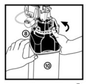
Grasp the empty Refill Bottle (1) with one hand and use the other hand to push the Green release latch on the Motor Assembly/Bottle Support (8) to the right (counterclockwise as seen from above).
