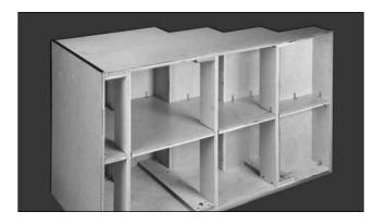
Attach all uprights with 2-1/4" hex bolts using 2 a washer under the bolt head and a washer against the locknut. Tighten securely with 9/16" socket wrench and 9/16" crescent wrench.
