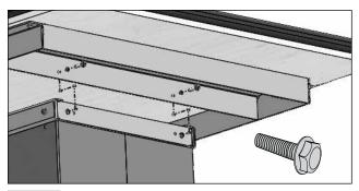
Working on just one end, elevate the top using help and align the holes on the top with the holes in the base. Insert the bolts removed from the shipping supports and finger tighten. DO NOT FULLY TIGHTEN.
