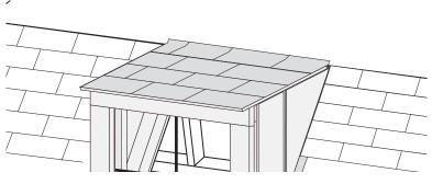
14. To shingle dormer, begin at the front of the roof panel and work backwards toward the roof pitch. Exposure should be 5", the same as the roof. Run the shingles all the way up until the dormer is covered. Shingle the remainder of the building.
