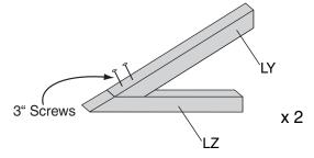
2. Using wall sub panel A, attach brackets as shown. Make sure sub panels are flush to the front and bottom of the brackets. Attach using
