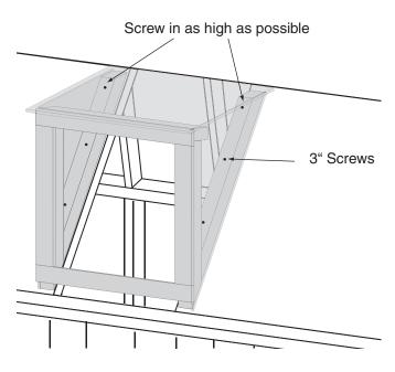
7. Center dormer over hole and attach using six 3" screws in the locations shown. Screws should be driven at a slight angle to be driven into the rafters.
