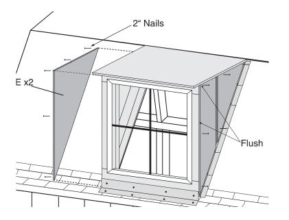
12. Attach the siding, E, as shown. Make sure the siding is flush to the front of the dormer and flush to the underside of the roof panel. Attach siding using six 2" nails per piece. Siding should leave about 3/8" gap above roof to allow for shingles.
