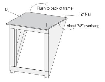
5. Attach the roof panel, D, using four 2" nails. The roof panel should be flush to the back and centered.
