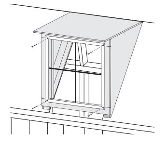
8. To attach window, center in the hole and fasten using four 1-1/4" screws in the predrilled corner holes.
