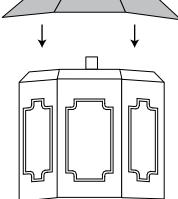
D: Center Cupola on roof, aligning Cupola corners with roof seams of gazebo roof and level. Pre-drill at a slight angle and anchor Cupola using (4) 2-1/2" screws into lower rafter.
