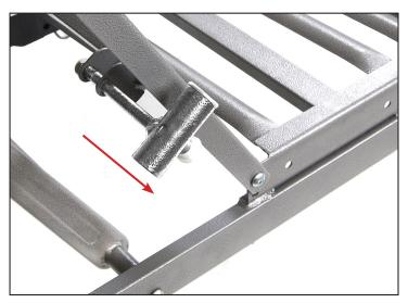
17. Turn the receptacle in order to receive the rail. Repeat for all four rail receptacles.
