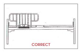
When installing bed rail, only place one (1) rail on bed per side.
