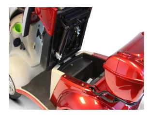
To release the seat latch, you need to start by inserting the key into the ignition. Without pushing inwards, turn the key counter clockwise (left). You should feel resistance while turning the key, until it hits a stopping point where it cannot turn anymore. If you do not feel any resistance, this means the key has been pushed inwards, which bypasses the seat latch release.
