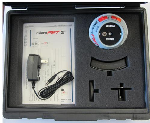
**Figure 1:** The microFET2™ device in supplied carrying case
