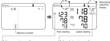
If the past reading was taken in TruRead mode. the " 3" symbol appears and the reading shown on the left is the average of 3 measurements.
