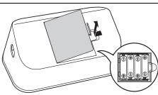
2. Insert 4 "AA" batteries as indicated in the battery compartment.
