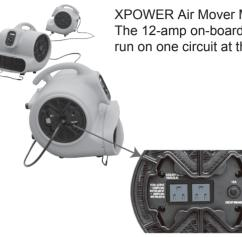
XPOWER Air Mover Model X-600A/P-600A are daisy chainable with a low 3.8 amp draw. The 12-amp on-board circuit breaker will allow two (2) additional same units to run on one circuit at the same time.
