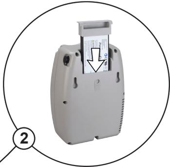
Insert Battery into back of EasyPulse TOC. (Ref. pg 7)
