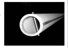
**Type T Core** (to fit Trane Company Roll Filter). Core is formed from 2-7/16" I.D. fiberboard tube. The tube contains a metal cup secured in each end recessed to a depth of 1-1/2" square.
